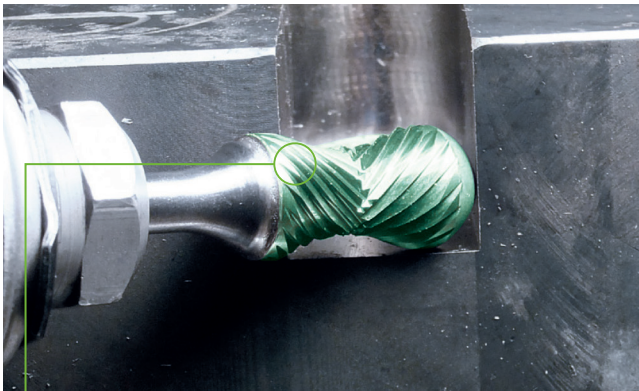
Interne Fase in SKM Form Internal chamfer with SKM shape
